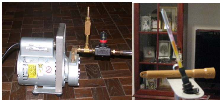
Figure 1. Hi-vol Pump Equipped with a Bypass Valve and Adsorption Tube Sampler.
