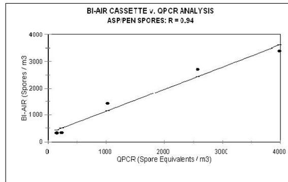
This graph illustrates the correlation between microscopic analysis and QPCR analysis performed directly on filter samples. Samples were collected on MCE filters using the Bi-Air cassette.
