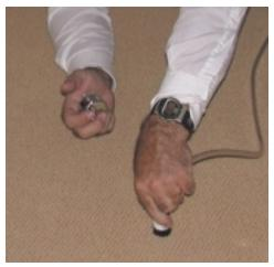
Figure 2 Using an open-face cassette to collect the sample from below the surface as well as from the surface of a soft-surface item.
