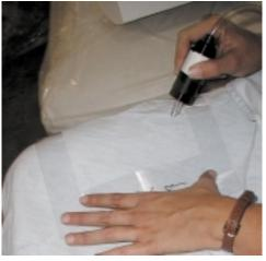
**Figure 1** Using a closed-face cassette to sample from the surface of a soft-surface item.
