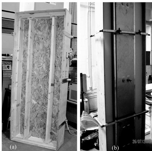
Figure 2. (a) View of a stud cavity; (b) View of sampling chamber installed on a wall assembly.
