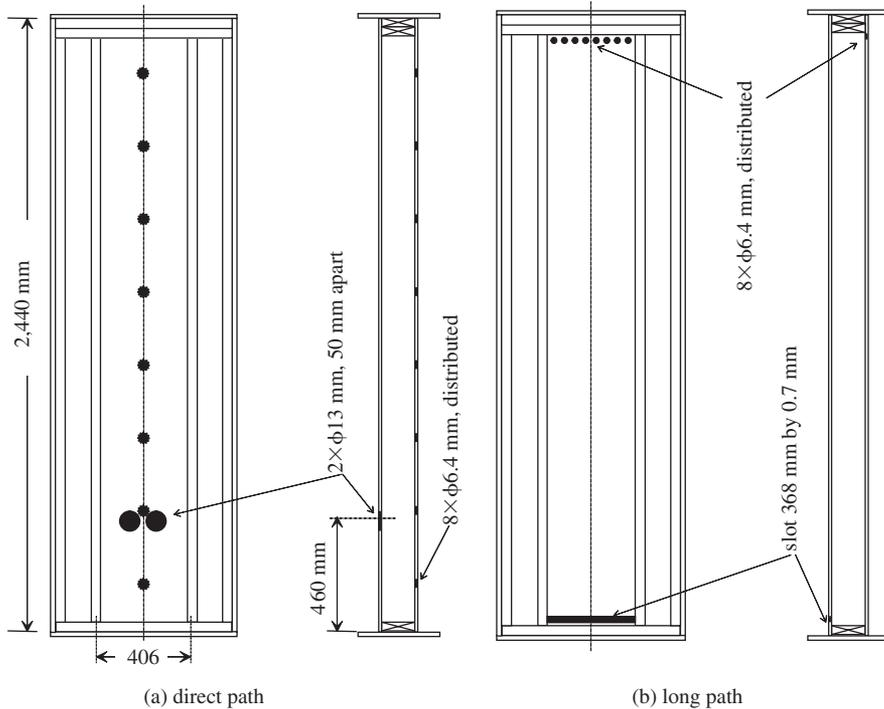
Figure 3. Air leakage openings and paths (not drawn to scale).
