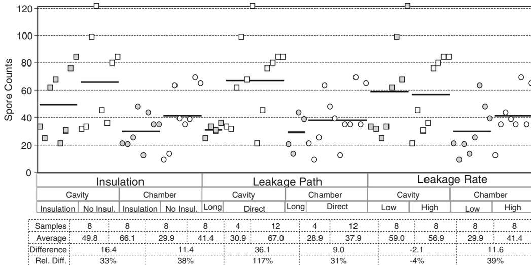
Figure 6. Influences of insulation, air leakage path and air leakage rate for data on wall assemblies with moldy studs and VBs.
