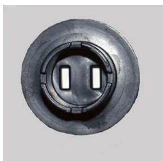
Figure 2. Bi-Air Cassette: Interior of the cowl showing the 1.7 mm x 5.5 mm dual sample traces with a total exposed filter area of 18.7 mm 2 .
