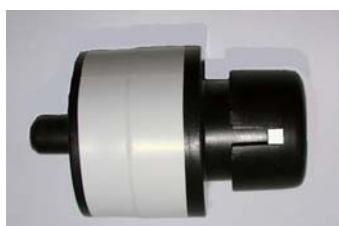
Figure 1. Bi-Air Cassette: Side view of the BA showing one of the four variable-width 3 mm x 3 mm sample inlets located in the side of the cowl.
